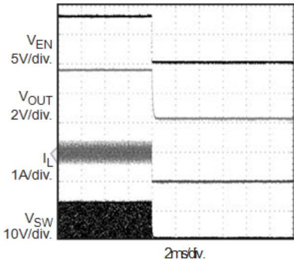
Figure 6. Shutdown through Enable
