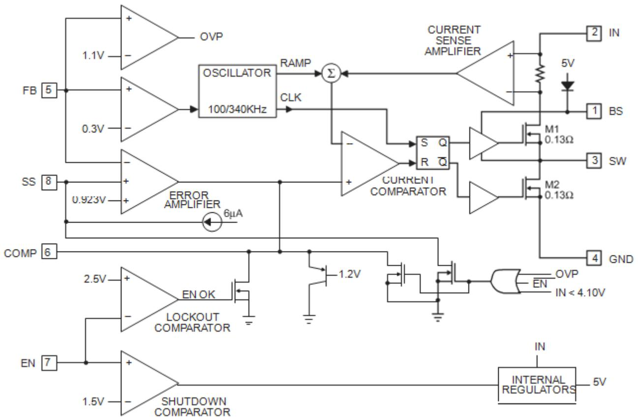
Figure 3 Function Block Diagram of TD1482A
