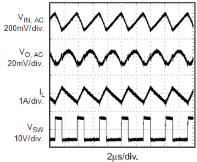
Figure 7. Heavy Load Operation
