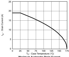
Maximum Avalanche Drain Current vs. Case Temperature
