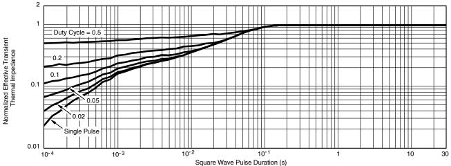
Normalized Thermal Transient Impedance, Junction-to-Case
