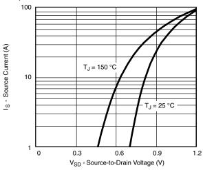
Source-Drain Diode Forward Voltage
