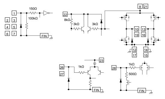
The equivalent circuit diagrams may be simplified or some parts of them may be omitted fo explanatory purposes. Absolute precision of the chip internal resistance is +/-30%.
