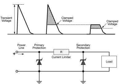
Fig. 8 - Secondary Protection Circuit
