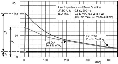
Fig. 6 - For ISO-7637-2 Test Conditions, the Standard Condition is a V<sub>S</sub> Range of 65 V to 87 V, and R<sub>i</sub> (Line Impedance) Range of 0.5  $\Omega$  to 4  $\Omega$
