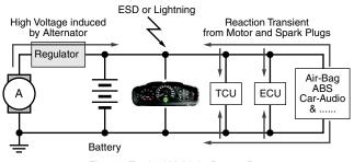
Fig. 4 - Typical Vehicle Power Bus
