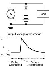
Fig. 5 - Output Voltage of Alternator in Load Dump Condition
