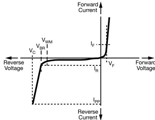
Fig. 3 - Parameters of Voltage and Current
