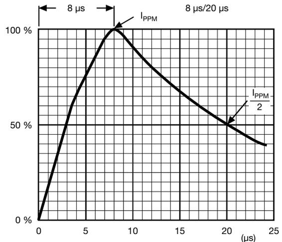
Fig. 2 - Test Waveform of TVS ESD
