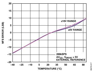
Figure 18. NFS Error vs. Temperature
