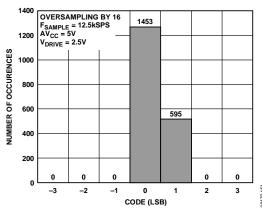
Figure 53. Histogram of Codes—OS × 16 (Two Codes)
