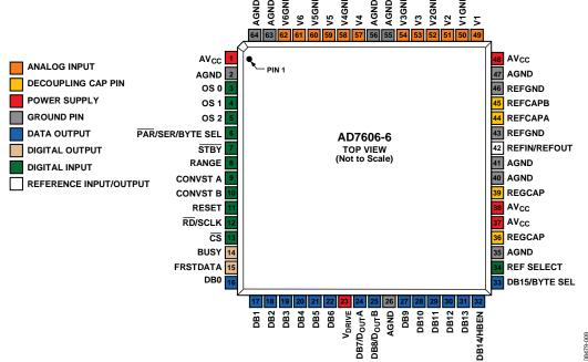
Figure 9. AD7606-6 Pin Configuration
