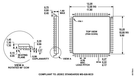
Figure 65. 64-Lead Low Profile Quad Flat Package [LQFP] (ST-64-2) Dimensions shown in millimeters
