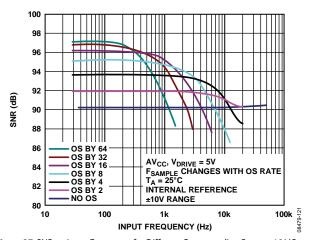
Figure 27. SNR vs. Input Frequency for Different Oversampling Rates,  $\pm 10\,\mathrm{V}$  Range
