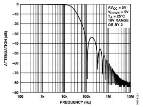
Figure 56. Digital Filter Response for OS 2
