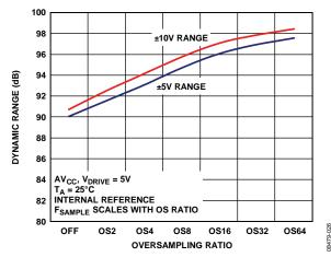
Figure 29. Dynamic Range vs. Oversampling Rate
