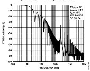
Figure 61. Digital Filter Response for OS 64
