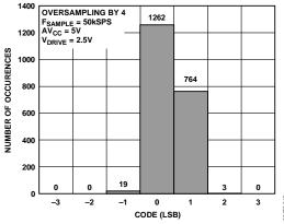
Figure 51. Histogram of Codes—OS × 4 (Four Codes)
