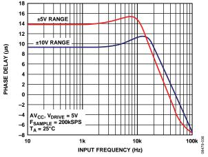
Figure 38. Analog Antialias Filter Phase Response
