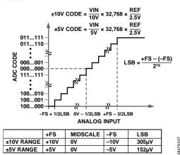
Figure 39. AD7606/AD7606-6/AD7606-4 Transfer Characteristics
