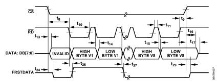
Figure 7. BYTE Mode Read Operation
