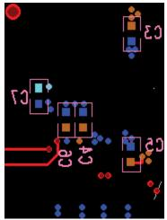
Figure 63. Bottom Layer Decoupling
