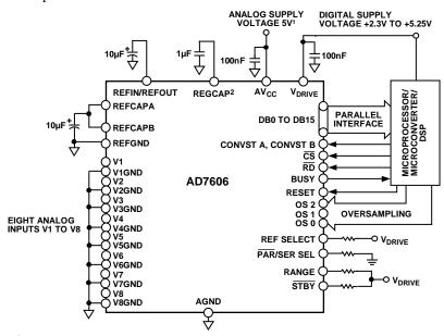
$^1\text{DECOUPLING}$  Shown on the AV $_{\text{CC}}$  PIN APPLIES TO EACH AV $_{\text{CC}}$  PIN (PIN 1, PIN 37, PIN 38, PIN 48). DECOUPLING CAPACITOR CAN BE SHARED BETWEEN AV $_{\text{CC}}$  PIN 37 AND PIN 38.
