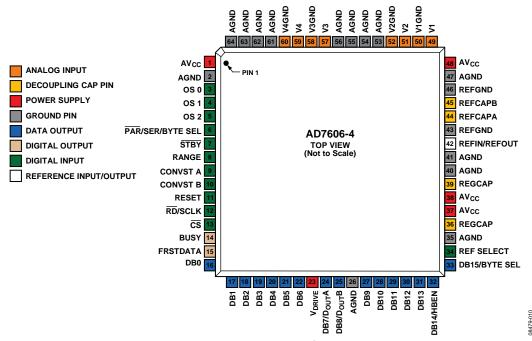
Figure 10. AD7606-4 Pin Configuration
