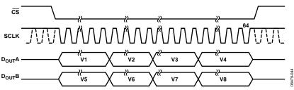
Figure 46. AD7606 Serial Interface with Two Dout Lines
