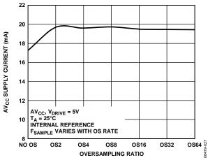
Figure 32. Supply Current vs. Oversampling Rate
