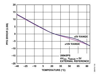
Figure 19. PFS Error vs. Temperature
