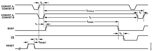
Figure 2. CONVST Timing—Reading After a Conversion
