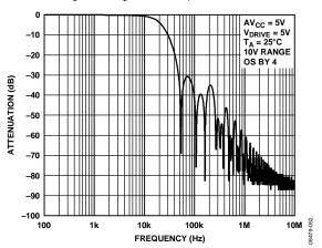
Figure 57. Digital Filter Response for OS 4
