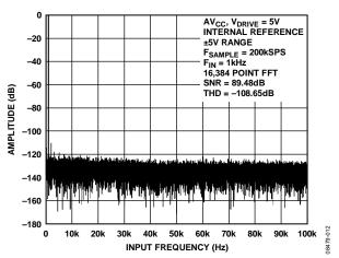
Figure 12. AD7606 FFT Plot, ±5 V Range
