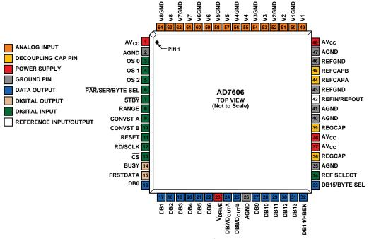
Figure 8. AD7606 Pin Configuration
