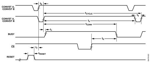
Figure 3. CONVST Timing—Reading During a Conversion
