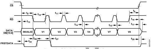
Figure 4. Parallel Mode, Separate  $\overline{\text{CS}}$  and  $\overline{\text{RD}}$  Pulses Rev. 0 | Page 9 of 36
