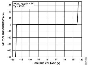
Figure 35. Input Protection Clamp Profile
