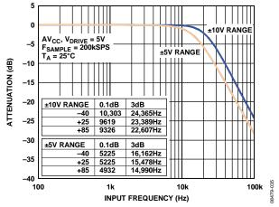
Figure 37. Analog Antialiasing Filter Frequency Response
