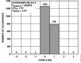
Figure 52. Histogram of Codes—OS × 8 (Three Codes)
