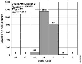
Figure 50. Histogram of Codes—OS × 2 (Four Codes)
