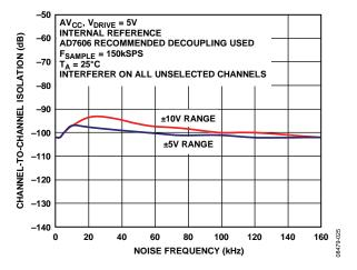
Figure 28. Channel-to-Channel Isolation
