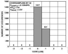
Figure 54. Histogram of Codes—OS  $\times$  32 (Two Codes)
