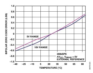
Figure 22. Bipolar Zero Code Error vs. Temperature
