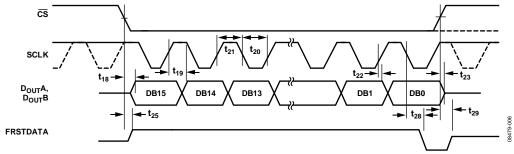
Figure 6. Serial Read Operation (Channel 1)
