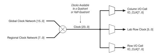
Figure 2–57. Hierarchical Clock Networks Per Quadrant
