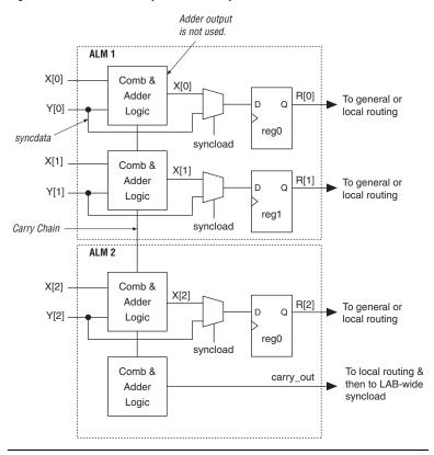
Figure 2–35. Conditional Operation Example
