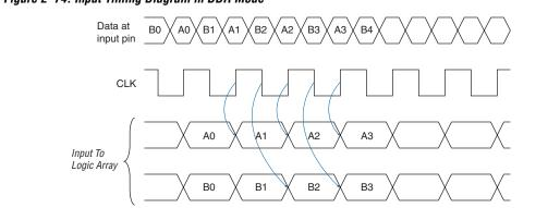
Figure 2–74. Input Timing Diagram in DDR Mode
