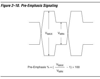
Pre-emphasis percentage is defined as  $(V_{MAX}/V_{MIN} - 1) \times 100$ , where  $V_{MAX}$  is the differential emphasized voltage (peak-to-peak) and  $V_{MIN}$  is the differential steady-state voltage (peak-to-peak).
