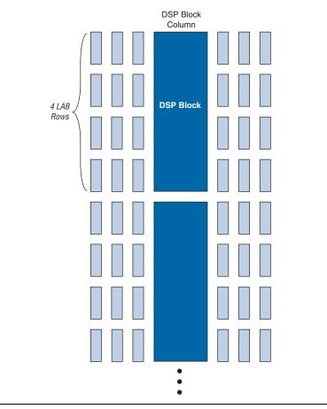
Figure 2–50. DSP Blocks Arranged in Columns
