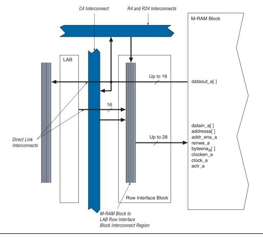
Figure 2–49. M-RAM Row Unit Interface to Interconnect
