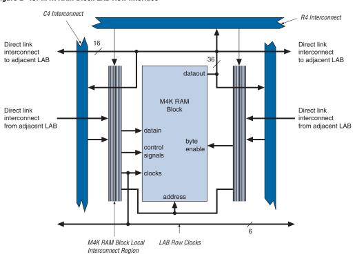
Figure 2-45. M4K RAM Block LAB Row Interface
