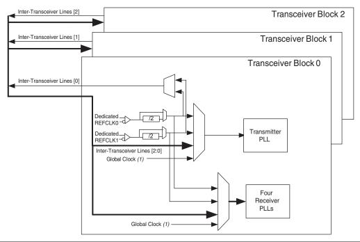
Figure 2–22. Input Reference Clock Sources
