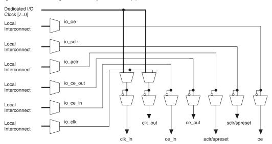
Figure 2–71. Control Signal Selection per IOE Note (1)
