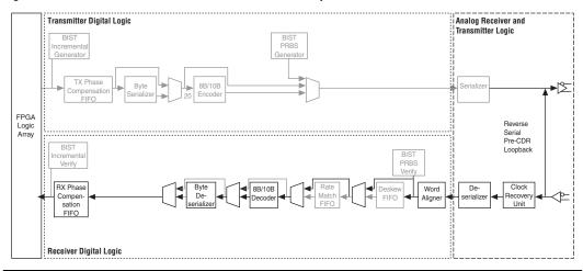
Figure 2–20. Arria GX Block in Reverse Serial Pre-CDR Loopback Mode
