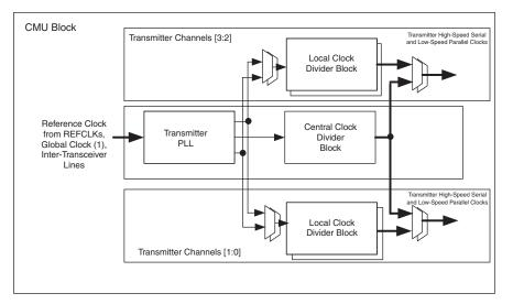
Figure 2–3 shows the block diagram of the clock multiplier unit.
