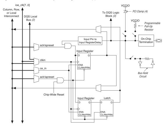
Figure 2–73. Arria GX IOE in DDR Input I/O Configuration Note (1)
