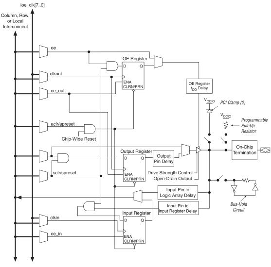
Figure 2–72. Arria GX IOE in Bidirectional I/O Configuration Note (1)
