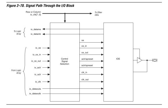
Each IOE contains its own control signal selection for the following control signals: oe, ce\_in, ce\_out, aclr/apreset, sclr/spreset, clk\_in, and clk\_out. Figure 2–71 illustrates the control signal selection.
