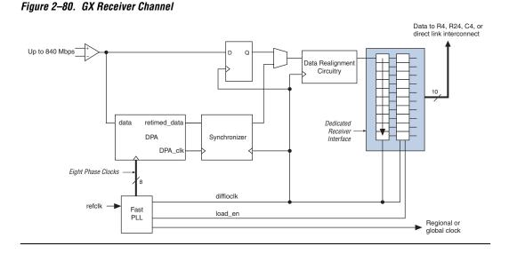
Figure 2–80 shows the block diagram of the Arria GX receiver channel.
