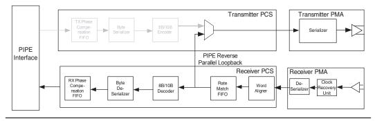
You can dynamically put the PCI Express (PIPE) mode transceiver in reverse parallel loopback by controlling the tx\_detectrxloopback port instantiated in the MegaWizard Plug-In Manager. A high on the
