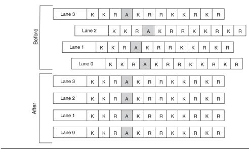
Figure 2–16. Before and After the Channel Aligner
