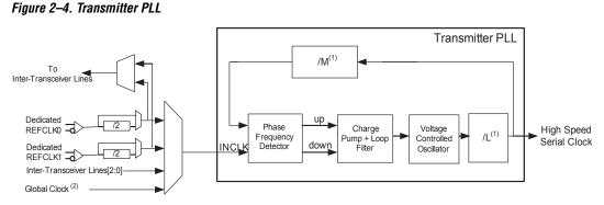
Figure 2–4 shows the block diagram of the transmitter PLL.
