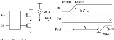
*Note to Figure 4–8:* (1) V<sub>CCINT</sub> is 1.12 V for this measurement.
