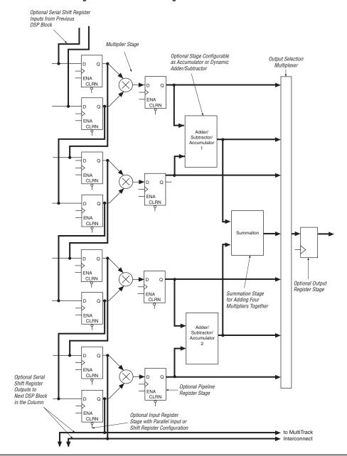
Figure 2–51. DSP Block Diagram for 18 × 18-Bit Configuration
