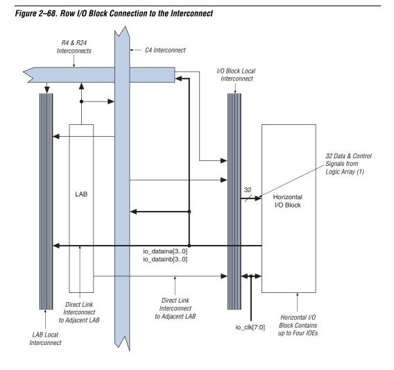
Figure 2–68 shows how a row I/O block connects to the logic array.
