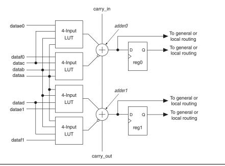
While operating in arithmetic mode, the ALM can support simultaneous use of the adder's carry output along with combinational logic outputs. In this operation, adder output is ignored. This usage of the adder with the combinational logic output provides resource savings of up to 50% for functions that can use this ability. An example of such functionality is a conditional operation, such as the one shown in Figure 2–35. The equation for this example is:
