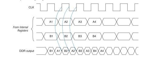
The Arria GX IOE operates in bidirectional DDR mode by combining the DDR input and DDR output configurations. The negative-edge-clocked OE register holds the OE signal inactive until the falling edge of the clock to meet DDR SDRAM timing requirements.
