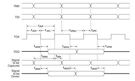
Table 4–123 shows the JTAG timing parameters and values for Arria GX devices.
