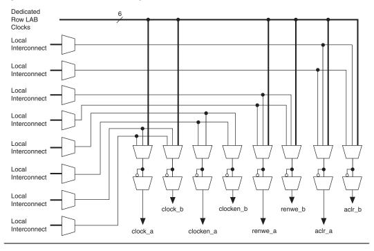
The R4, C4, and direct link interconnects from adjacent LABs drive the M4K RAM block local interconnect. The M4K RAM blocks can communicate with LABs on either the left or right side through these row resources or with LAB columns on either the right or left with the column
