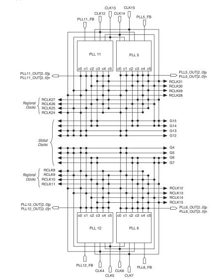
*Figure 2–64. Global and Regional Clock Connections from Top and Bottom Clock Pins and Enhanced PLL Outputs Note (1)*
