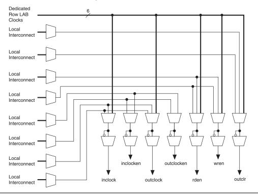
The RAM blocks in Arria GX devices have local interconnects to allow ALMs and interconnects to drive into RAM blocks. The M512 RAM block local interconnect is driven by the R4, C4, and direct link interconnects from adjacent LABs. The M512 RAM blocks can communicate with LABs on either the left or right side through these row interconnects or with LAB columns on the left or right side with the column interconnects. The
