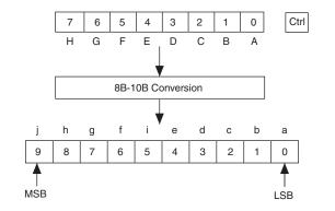
During reset (tx\_digitalreset), the running disparity and data registers are cleared and the 8B/10B encoder outputs a K28.5 pattern from the RD- column continuously. Once out of reset, the 8B/10B encoder starts with a negative disparity (RD-) and transmits three K28.5 code groups for synchronizing before it starts encoding the input data or control character.
